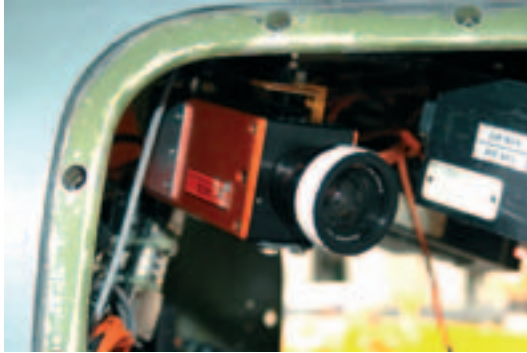
S-EM positioned inside pod
