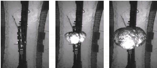
Sub Sea recording of blast with S-VIT camera, recording taken @ 1000fps
